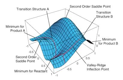
Figure 6.1: A model potential energy surface illustrating important stationary points and curves. (from Jack Simons:Introduction to theoretical chemistry)
