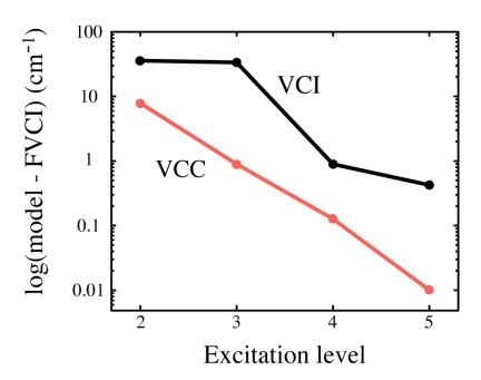
Figure 6.3: Comparison of vibrational excitation energies between VCI[n] and VCC[n]. Errors relative to FVCI in  $cm^{-1}$  for the eight lowest fundamental vibrations of ethylene for different truncation of the excitation space determined by n. (Seidler and Christiansen).
