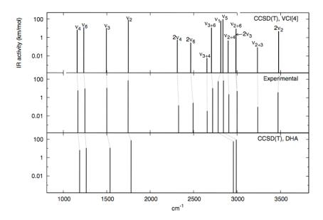
Figure 6.1: Comparison of formaldehyde vibrational excitation energies in experiment, the double harmonic approximation, and VCI[4] using a relative accurate potential) (Seidler and Christiansen, 2007).
